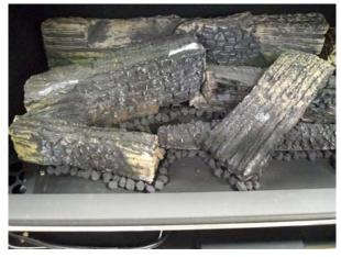
4) Line up some of the coals that have been supplied with this appliance, along the burner holes in front of the logs.
